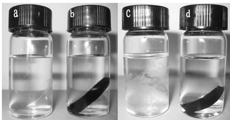
Fig. 8. Photographs of pure chitosan (a, c) and CS/GO-3 (b, d) films immersed in distilled water for 10 min (a, b) and 30 days (c, d).
